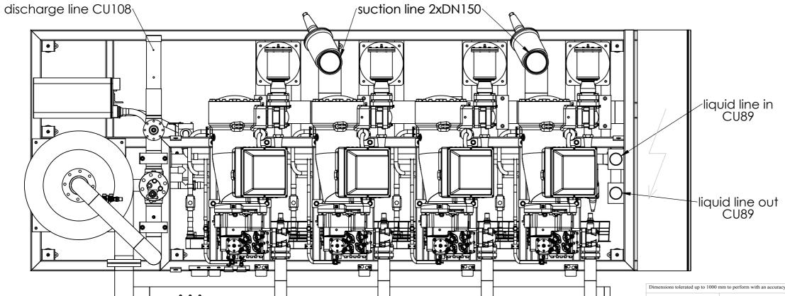
Dimensions tolerated up to 1000 mm to perform with an accuracy of +/- 1 mm, dimensions greater than 1000 mm with an accuracy of +/- 2 mm. The guidelines do not apply hole diameters.
